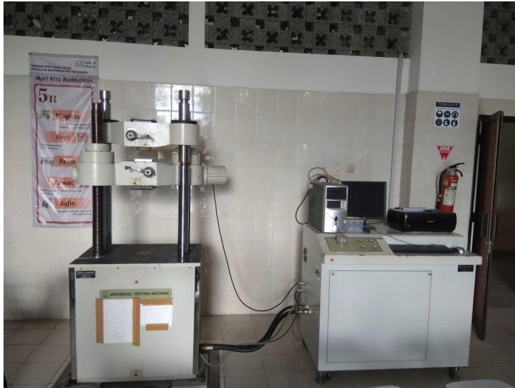
Gambar 3.11. Micro-computer Universal Testing Machine (UTM)
